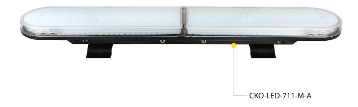
The above photo shows the bolt-mounted version of this product. The magnetically mounted version is aesthetically identical, with the only difference being the fixture used for mounting.
