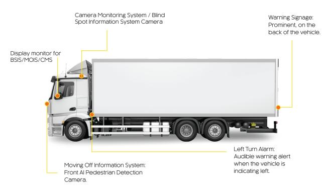
\*for left hand drive vehicles blind spot location and equipment positioning is adjust accordingly
